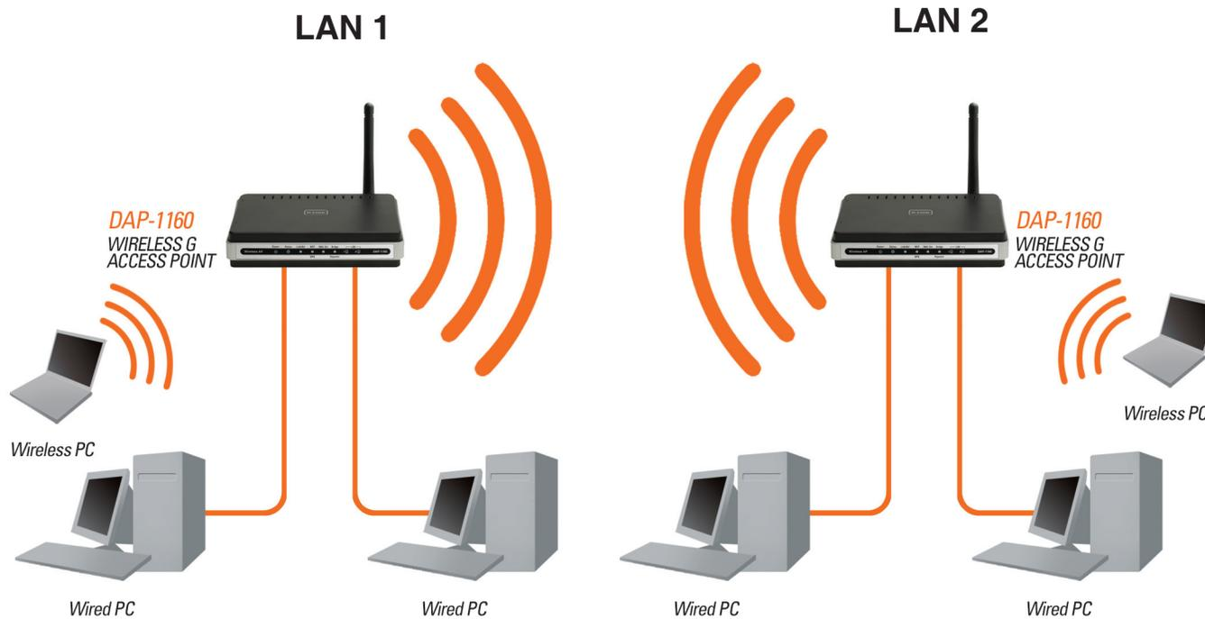
**Connecting Two Separate LANs Together Through Two DAP-1160 Units
