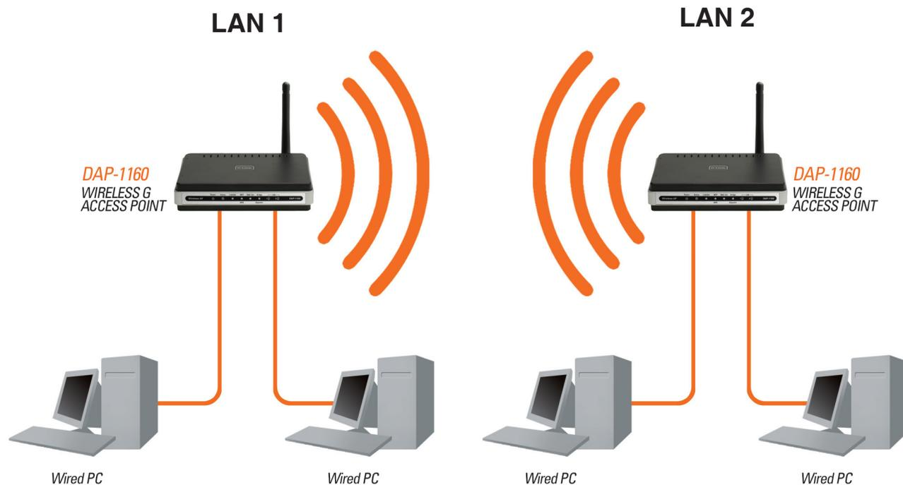
**Connecting Two Separate LANs Together Through Two DAP-1160 Units
