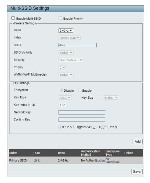
Encryption: When you select Open System, toggle between Enable and Disable. If Enable is selected, the Key Type, Key Size, Key Index
