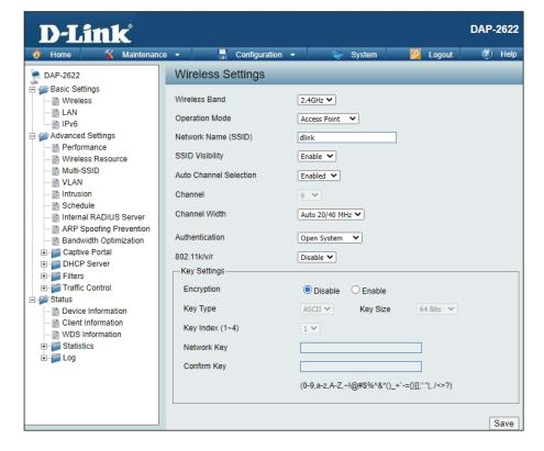
**Channel:** To change the channel, first toggle the *Auto Channel Selection* setting to **Disable**, and then use the drop-down menu to make the desired selection.
