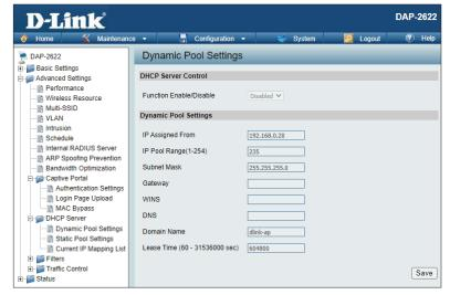
Subnet Mask: All devices in the network must have the same subnet mask to communicate. Enter the subnet mask for the network here.
