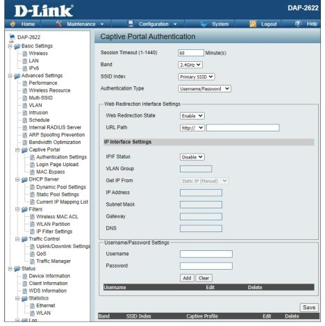
Get IP From: Static IP (Manual) is chosen here. Choose this option if you do not have a DHCP server in your network, or if you wish to assign a static IP address to the DAP-2622. When Dynamic IP (DHCP) is selected, the other fields here will be grayed out.
