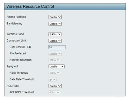
**User Limit:** Set the maximum amount of users that are allowed access (zero to 64 users) to the device using the specified wireless band. The default setting is **20**.
