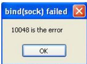
**A1:** This Windows error will occur if the Internet Camera is connected to a computer that is not properly configured with a valid IP address. Turn off DHCP from the Network Settings in Windows and configure the computer with a valid IP address or connect the camera to a router with DHCP enabled.
