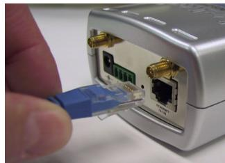
If you are connecting the **DCS-2100+** to a **802.11b wireless** Ethernet network, attach the two wireless antennas to the antenna connectors on the back panel of the **DCS-2100+**.
