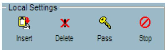
**Insert** – To add cameras to the camera list, specify the IP address and port, click the **Insert** button. The program will try to connect to the **DCS-2100+**. If the connection succeeds, the admin password of the remote **DCS-2100+** camera is required. If you provide the correct password, the camera will be inserted in the list.
