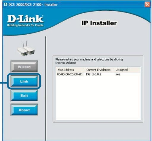
After you click on the **Link** button, **IP Installer** will automatically open your Internet browser to the IP Address of the **DCS-2100+**, in this example it is: <http://192.168.0.146> Your **DCS-2100+** may have a different IP Address.
