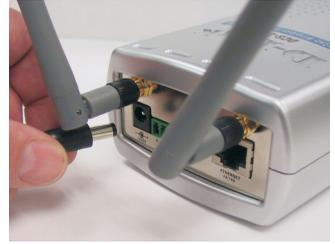
When you have a proper connection, the **LED** (Light Emitting Diode) on the front of the camera will turn from red to green. The light may blink on and off and your computer may show an intermittent loss of connectivity, this is normal until you have configured your camera.
