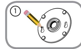
2. Depending on the material of the wall or ceiling, use proper tools to drill two holes or screws where you marked. If the wall is made out of concrete, drill the holes first, insert the plastic anchors and then the screws.
