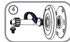
5. Adjust the angle of the camera as desired, then tighten the collar on the camera stem to lock it in place.
