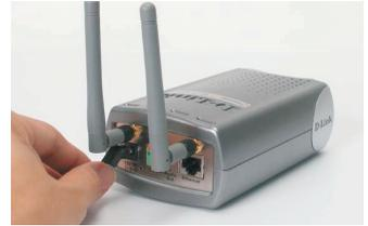
When you have a proper connection, the **LED** (Light Emitting Diode) on the front of the camera will turn from red to green. The light may blink on and off and your computer may show an intermittent loss of connectivity if you have it directly connected to the camera. This is normal until you have configured your camera.
