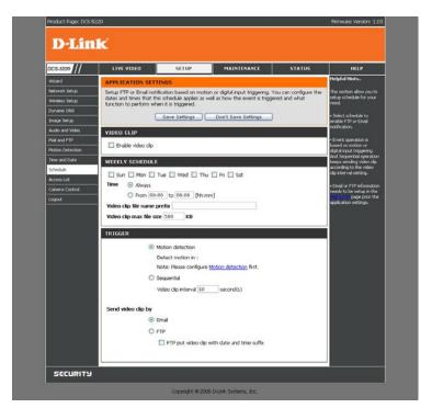
Detect Motion in: Check the motion detection window(s) to enable motion triggering. The window(s) can be created in the
