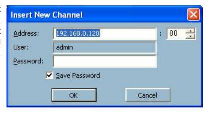
Once the camera is added, you will see the IP address of the camera and also the port that is opened on the camera (port 80 in this example). The selected camera has been added to the selection list.
