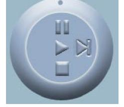
**Forward:** This button is only valid when the displaying video sequence is paused. It will display the next frame in that period when you click on the "Forward" button one time.
