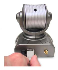
Attach the external power supply to the DC power input connector located on the Internet Camera's back panel (labeled DC 12V) and connect it to an AC power outlet.
