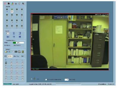
To view an individual camera from the multi-camera layout, double-click on the desired display window. You will see that the size of the display window is the same as the one-channel layout. Clicking the Back button in the upper-left corner of the video area will switch to the previous selected multi-camera layout.
