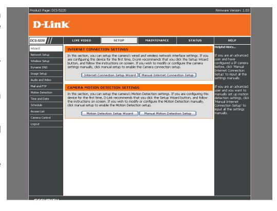
The Setup page provides the following configuration options: Wizard, Network Setup, Wireless Setup, Dynamic DNS, Image Setup, Audio and Video, Mail and FTP, Motion Detection, Time and Date, Schedule, Access List, Camera Control, and Logout.
