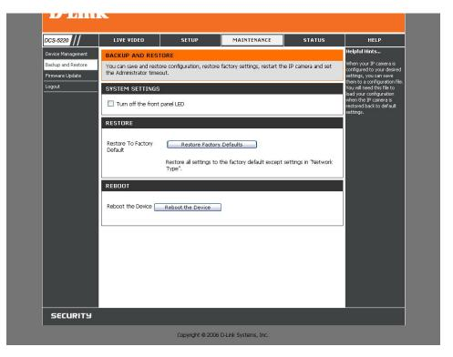
Click Apply on this screen to restore the factory default settings. After confirmation, the system will restart and require the DCC program to locate the IP address of the DCS-5220.
