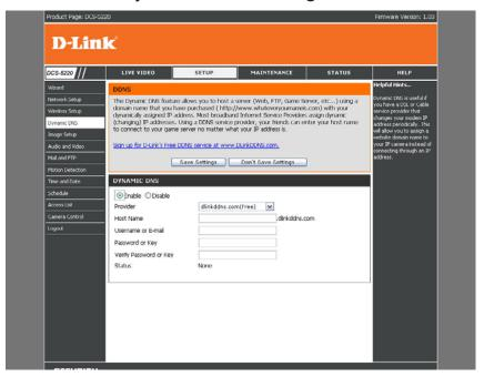
Dynamic DNS (DDNS): Dynamic DNS (Domain Name Service) is a method of keeping a domain name linked to a changing (dynamic) IP address. With most Cable and DSL connections, you are assigned a dynamic IP address and that address is used only for the duration of that specific connection. With the DCS-5220, you can set up your DDNS service and the DCS-5220 will automatically update your DDNS server every time it receives a different IP address.
