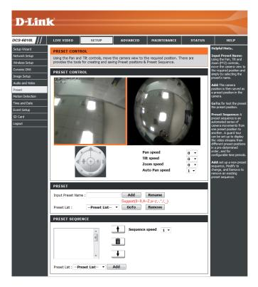
Preset Sequence: This section allows you to create a preset sequence, which automatically moves the camera's view between a set of preset views.
