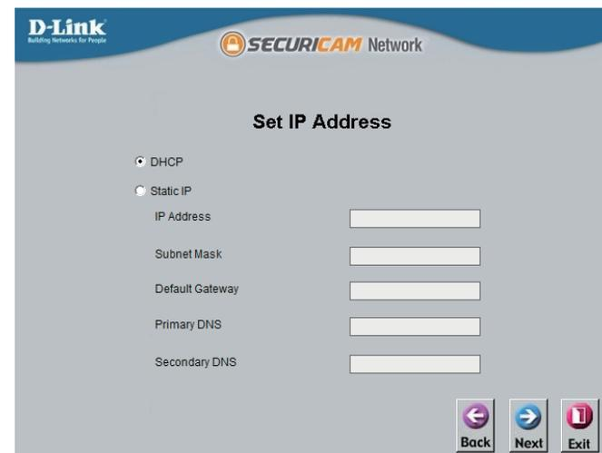
The screenshot shows the 'Set IP Address' screen. It has two radio buttons: 'DHCP' (selected) and 'Static IP'. Below are five input fields: 'IP Address', 'Subnet Mask', 'Default Gateway', 'Primary DNS', and 'Secondary DNS'. At the bottom right are 'Back', 'Next', and 'Exit' buttons.
