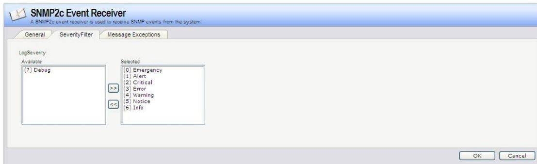
Figure 5: SNMP2c Event Receiver configuration, SeverityFilter tab
