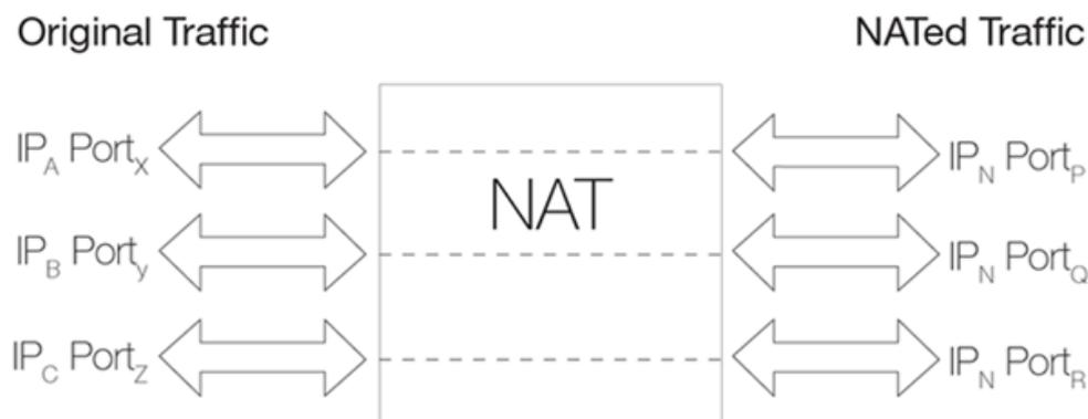
In the illustration above, three connections from IP addresses *A*, *B* and *C* are NATed through a single single source IP address *N*. The original port numbers are also changed.
