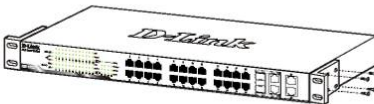
Figure 2.2 – Attach the mounting brackets to the Switch
