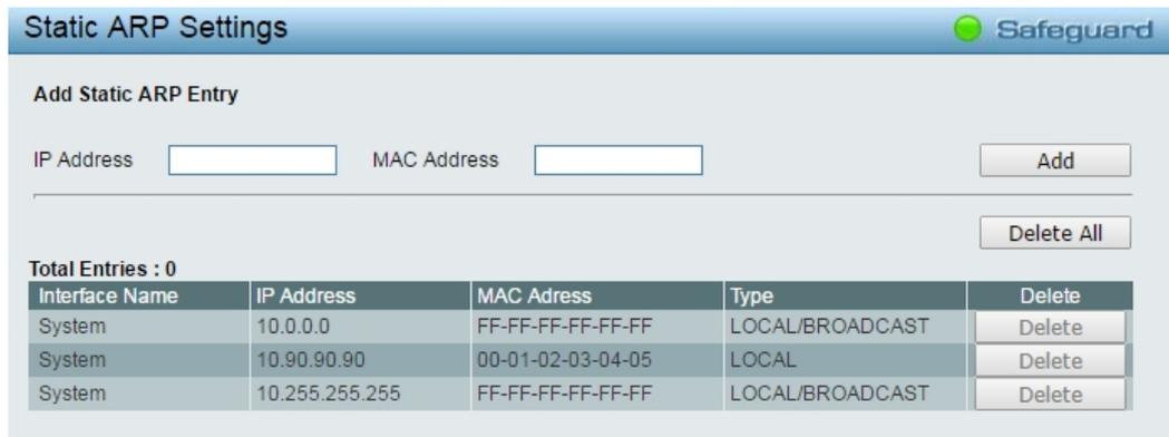
Figure 4.87 – L3 Functions > ARP > Static ARP Settings
