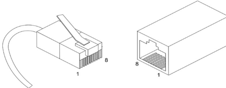
**Figure A-1. RJ-45 Pin Allocation**
