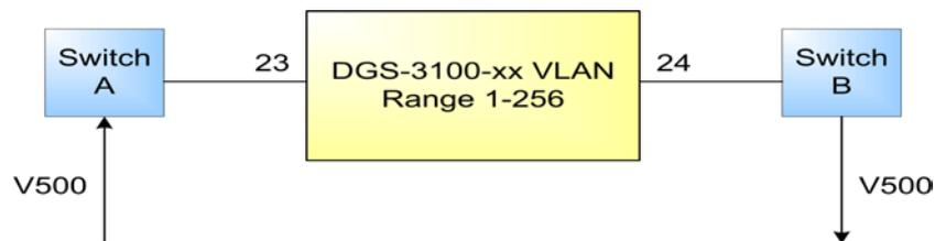
Figure 3–11. VLAN Trunking example between 2 switches
