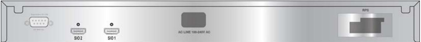
**Figure 1-4. DGS-3100 24P/48P Rear Panel View**
