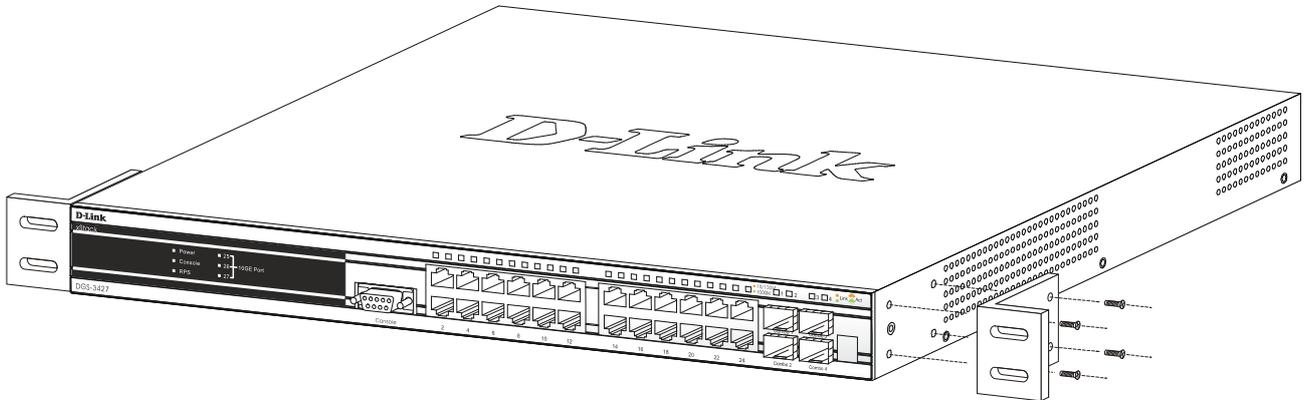
**Figure 2- 17. Fasten mounting brackets to Switch**
