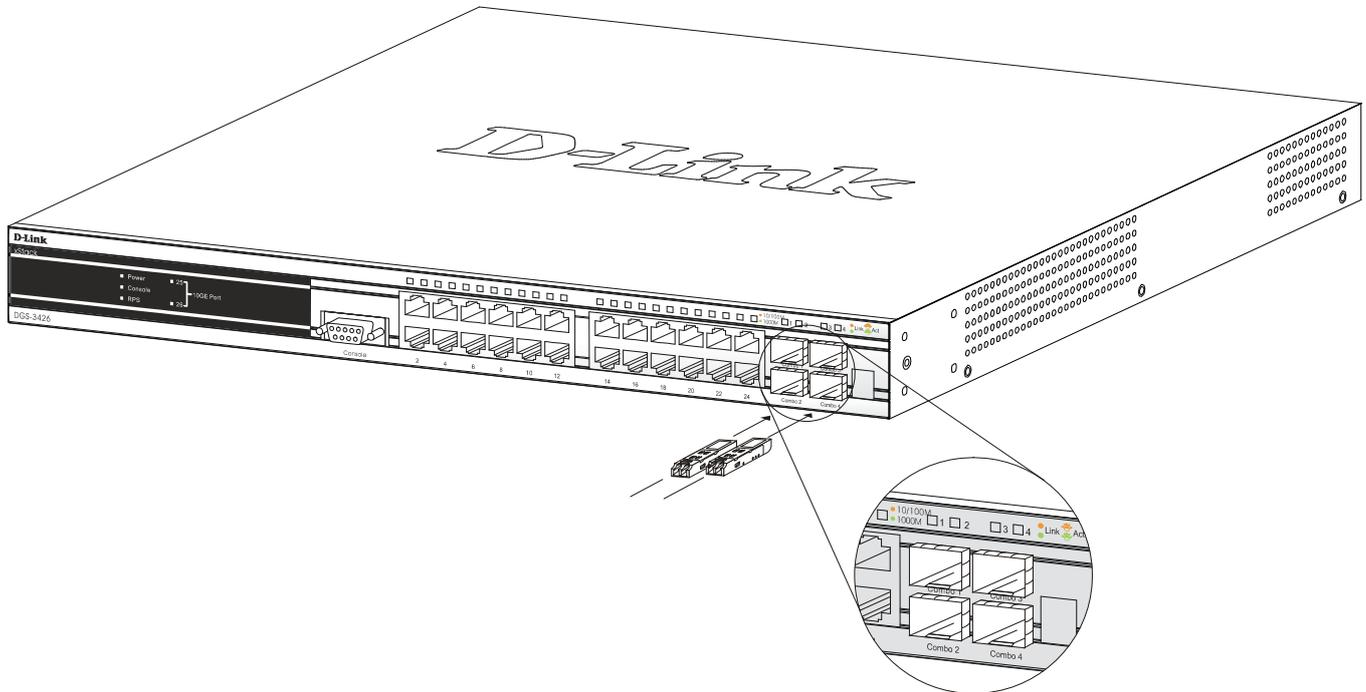
**Figure 2- 19. Inserting the fiber-optic transceivers into the DGS-3426**
