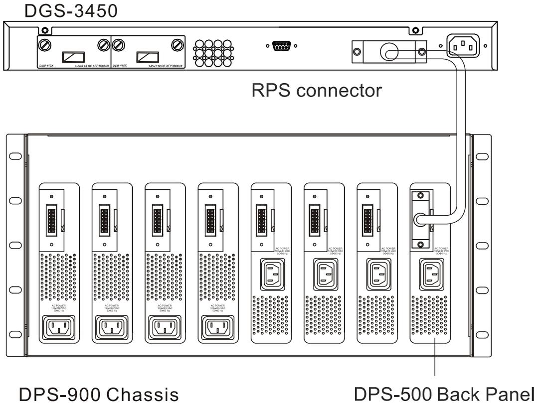
Figure 2- 24. The DGS-3450 with the DPS-500 chassis RPS
