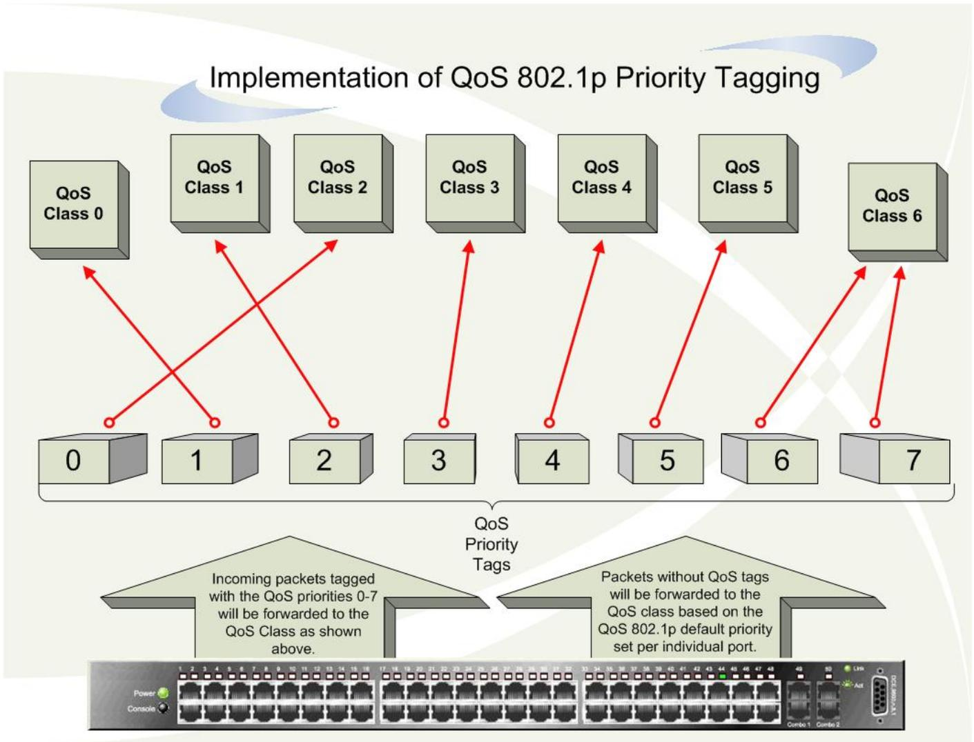
**Figure 8- 1. An Example of the Default QoS Mapping on the Switch**
