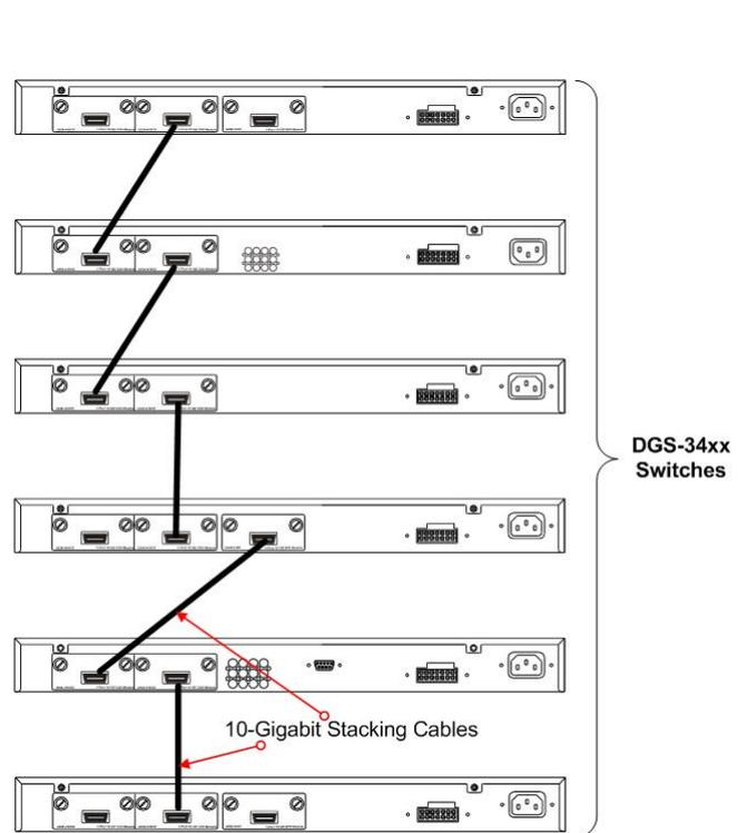
**Figure 6- 10. Switches stacked in a Duplex Chain**
