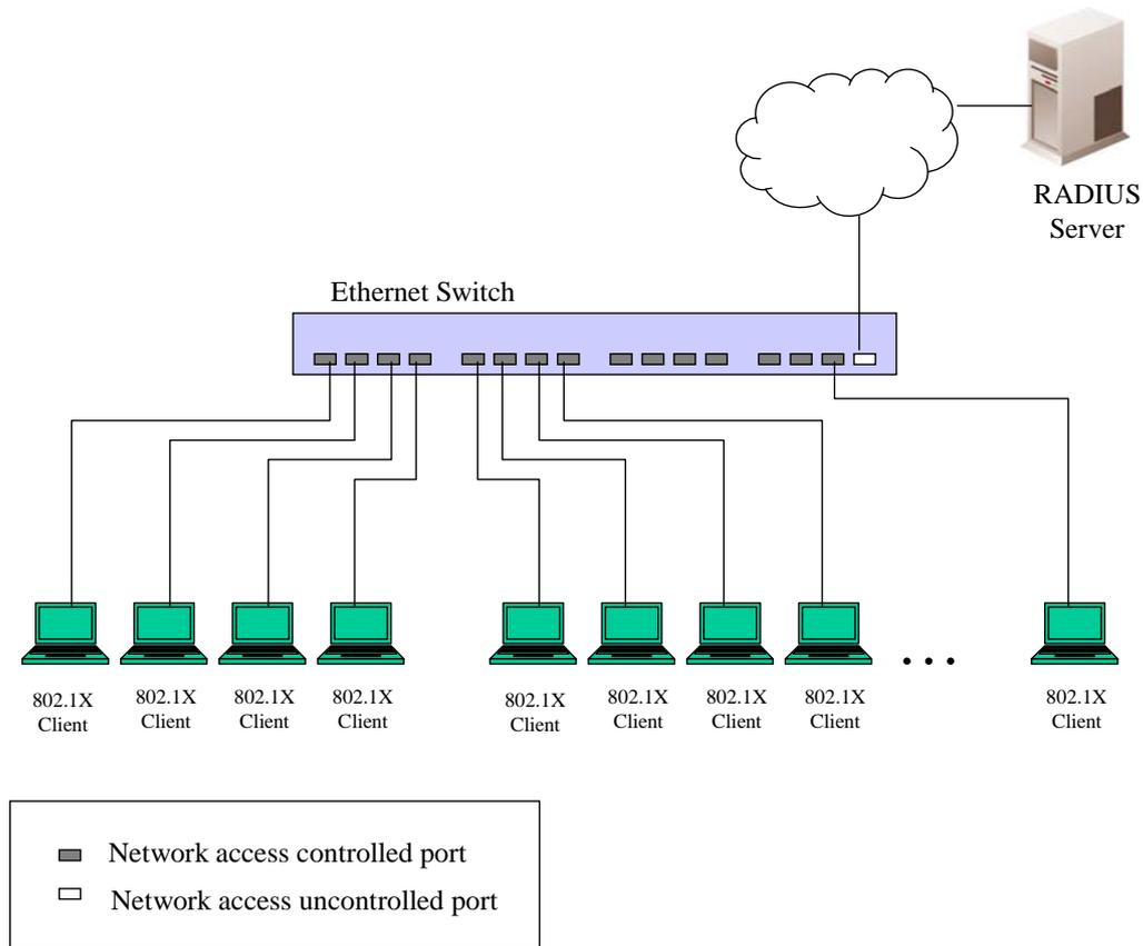
**Figure 10- 11. Example of Typical Port-Based Configuration**
