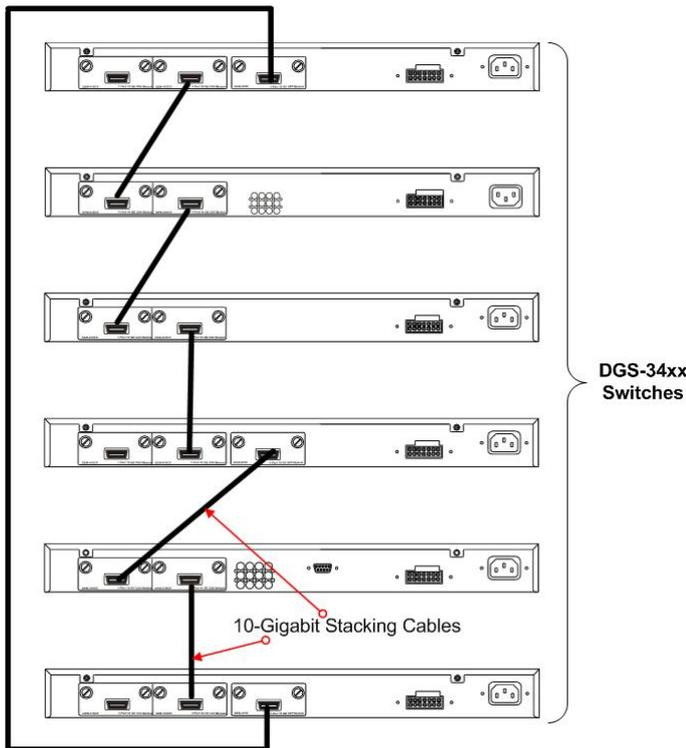
**Figure 6- 9. Switches stacked in a Duplex Ring**
