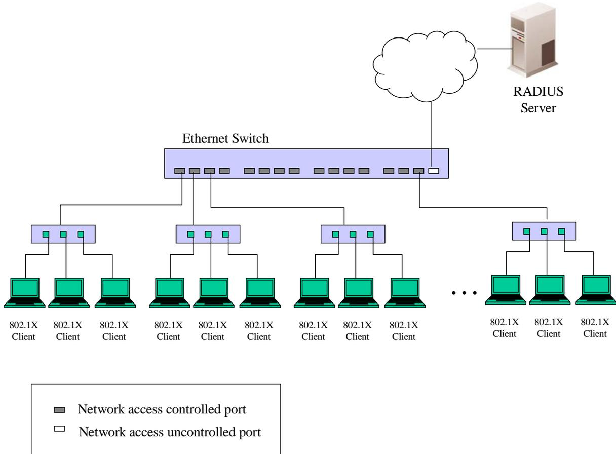
**Figure 10- 12. Example of Typical MAC-Based Configuration**
