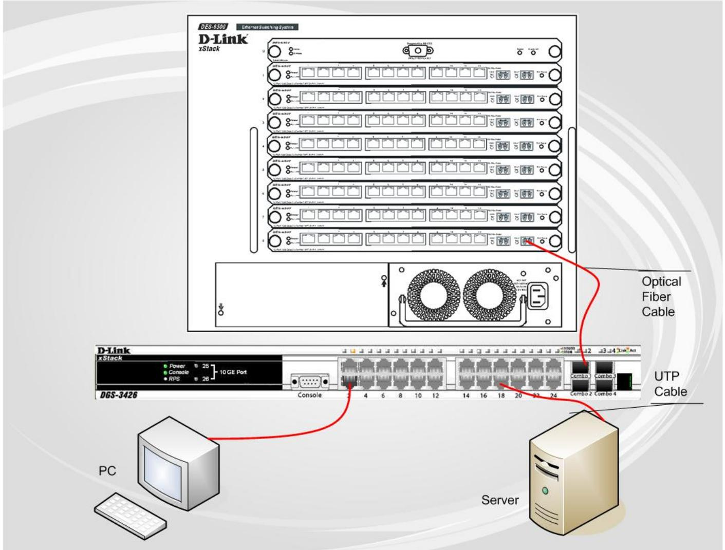
Figure 3- 3. DGS-3400 uplink connection to a server, PC or switch stack.
