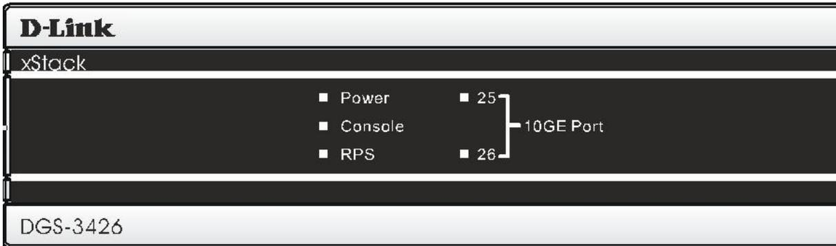
Figure 2- 7. LED Indicators on DGS-3426
