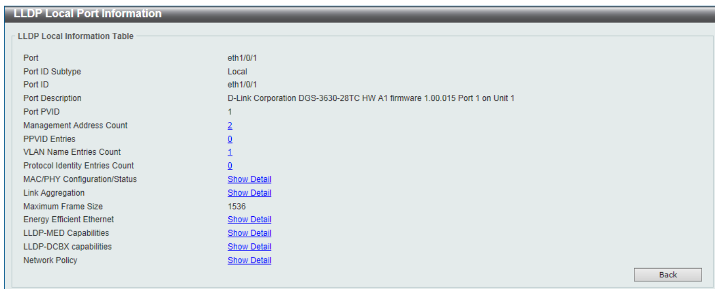
Figure 5-105 LLDP Local Port Information (Show Detail) Window
