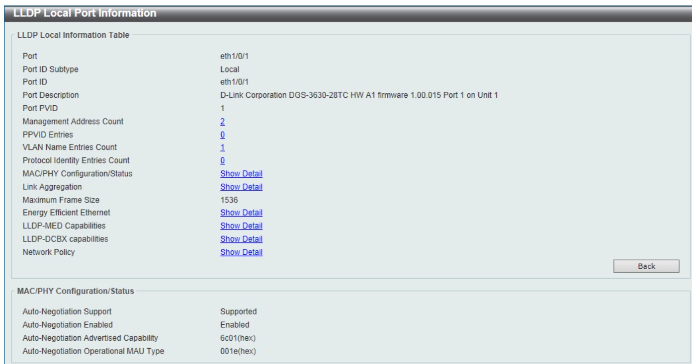
Figure 5-106 LLDP Local Port Information (Show Detail) Window
