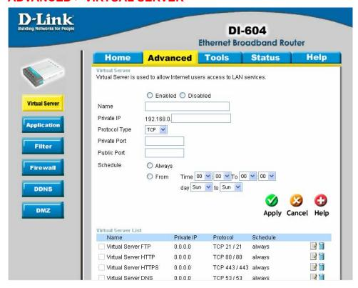
The DI-604 can be configured as a virtual server so that remote users accessing Web or FTP services via the public IP address can be automatically redirected to local servers in the LAN network.
