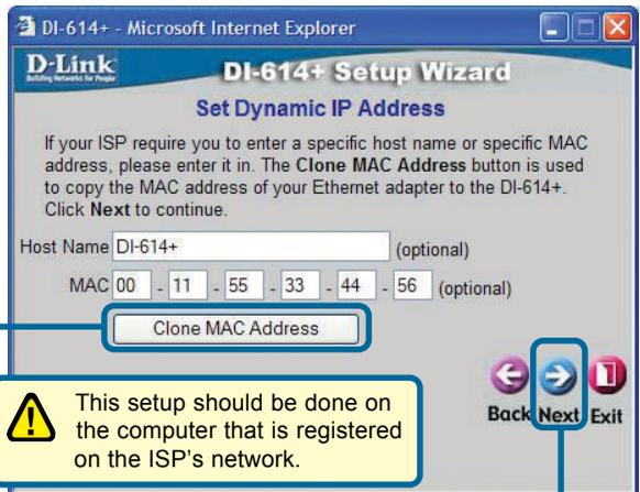
Click the **"Clone MAC Address"** button to automatically copy the MAC address of the network adapter in your computer. You can also manually type in the MAC address.
