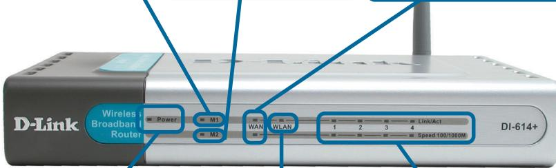
**POWER LED** – a solid light indicates a proper connection to the power supply.
