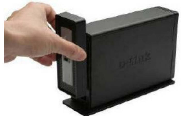
3. Insert a 3.5" SATA hard drive into an available drive bay. Make sure to align the drive connector to the SATA connector on the bottom edge inside the drive bay of the DNS-313. Gently push the drive in until it connects.
