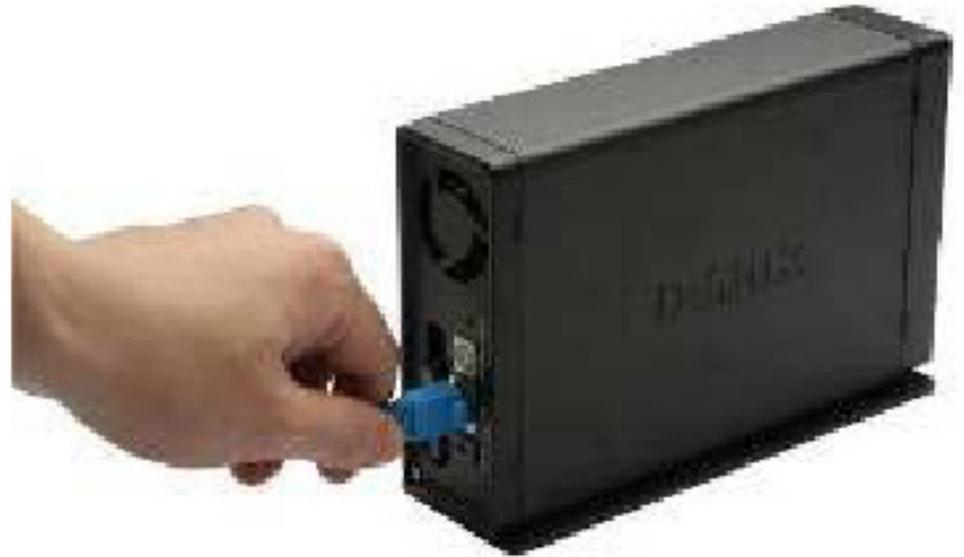
6. Connect the supplied power adapter to the power receptacle.
