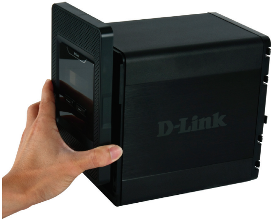
Detach the front cover of the NAS
