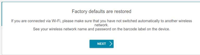
If you perform initial configuration of the router via Wi-Fi connection, please make sure that you are connected to the wireless network of DSL-224 and click the **NEXT** button. Then click the **START** button.
