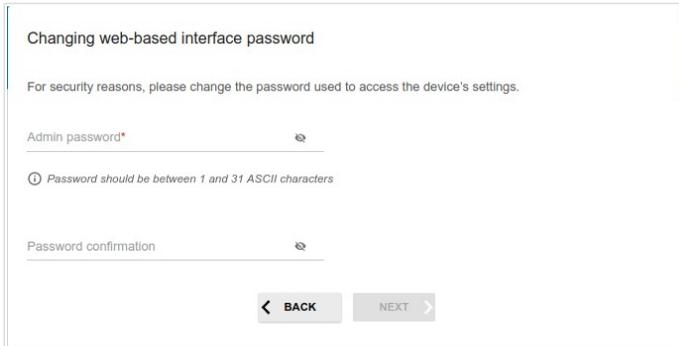
**!** Remember or write down the new password for the administrator account. In case of losing the new password, you can access the settings of the router only after restoring the factory default settings via the hardware **RESET** button. This procedure wipes out all settings that you have configured for your router.
