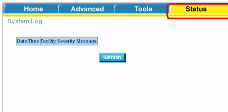
**NOTE:** When you click on the **View System Log** button, the System Log screen that you access will be located under the **Status** section (see screen on left). To return to the previous screen to configure system log, remember to click on the **Tools** tab (located on top row) first and then click on **Remotelog**.
