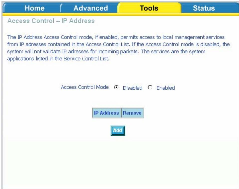
To assign the IP address of the management station that is permitted to access the local management services, enter the IP address in the box and click on the **Apply** button.
