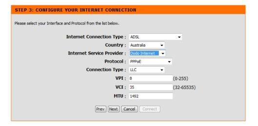
In this step, the user can configure the Internet connection settings used by this router.
