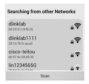
3. If your mobile device has saved the router's wireless password, it will be automatically associated to your router, otherwise D-Link One Touch will pop-up a password dialog, you need enter correct Wi-Fi password and tap **Connect** button associate your router.
