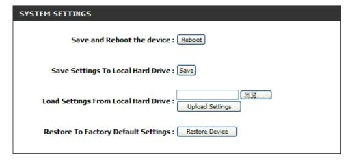
button. If the admin's password is lost you can no longer manage the DSL-2877AL. Use the restore switch at the back of the device. Warning! When you select to restore the Default Settings you will lose any settings defined before.
