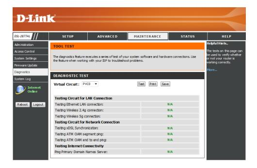
In this section diagnostic tests are performed to test the connection to the **Local Network** interface and **DSL Service Provider**. This test will include testing the **Ethernet**, **Wireless** connections, **ATM OAM**, and **Internet Connectivity** of this router.
