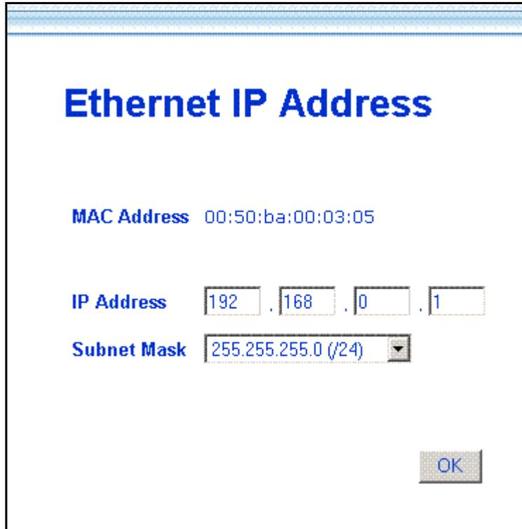
Figure 4- 3. Ethernet IP Address Menu
