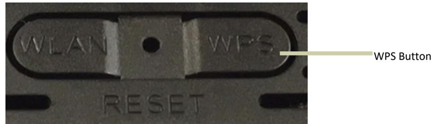
**Step 2** - Within 2 minutes, press the WPS button on your wireless device (or launch the software utility and start the WPS process).
