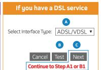
**Note:** If a red message appears stating "Connection failure" please confirm that the cable from the LAN port on the Fibre ONT device has been inserted into the Blue WAN port on the back of the router.
