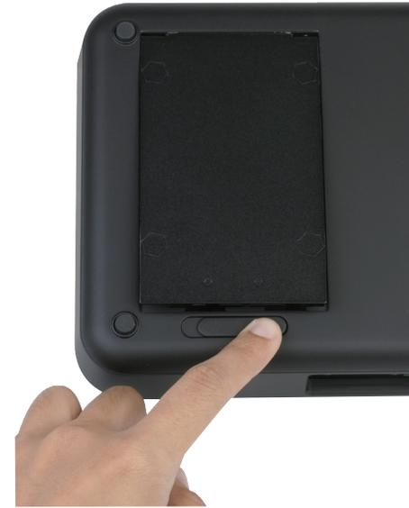
Insert the hard drive as shown and push it into the drive connector firmly.
