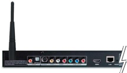
**Note:** You may have an Ethernet cable plugged into the unit and have the wireless antenna connected. Neither will interfere with the other, but only one network can be accessed at a time (wired or wireless). The network connection type is selected in the Setup Wizard and can also be changed by going to the Setup Menu. To access the Setup Menu, press the **SETUP** button on the remote control.
