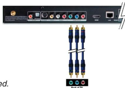
The **VIDEO OUT** button on the remote control toggles between the composite/S-Video output, the component video output, and the HDMI output. If component connectors are used but not selected, the screen will be tinted blue.
