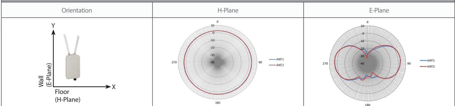
5 GHz Antenna Wall/Pole Mounted
