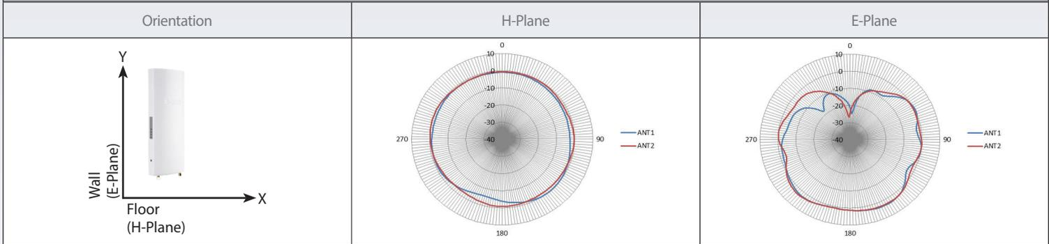
5 GHz Antenna Wall/Pole Mounted
