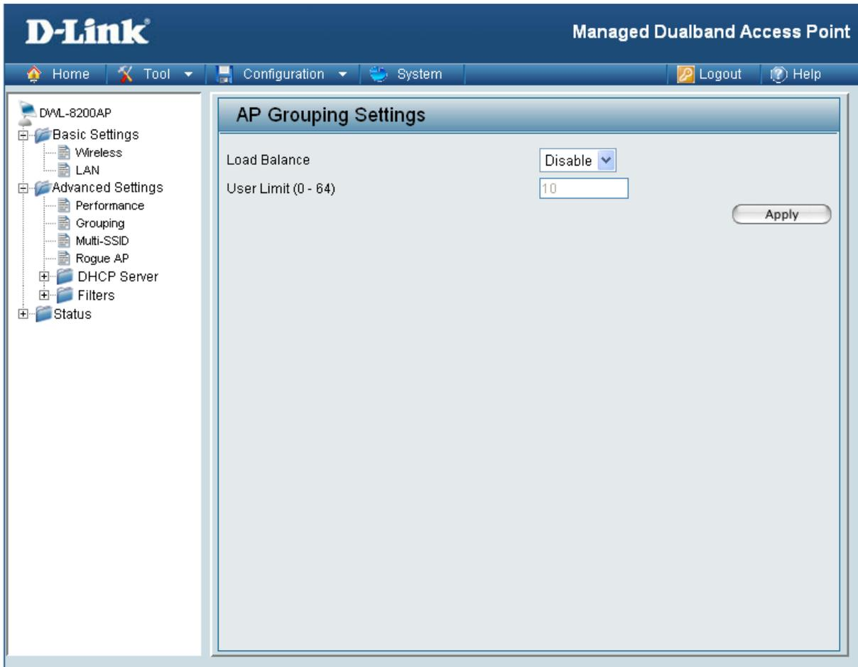
**Load Balance:** When **Enabled**, you allow several **DWL-8200APs** to balance wireless network traffic and wireless clients among **DWL-8200APs** in the network. Assign each access point a different **non-overlapping channel** (e.g., 1, 6, 11).
