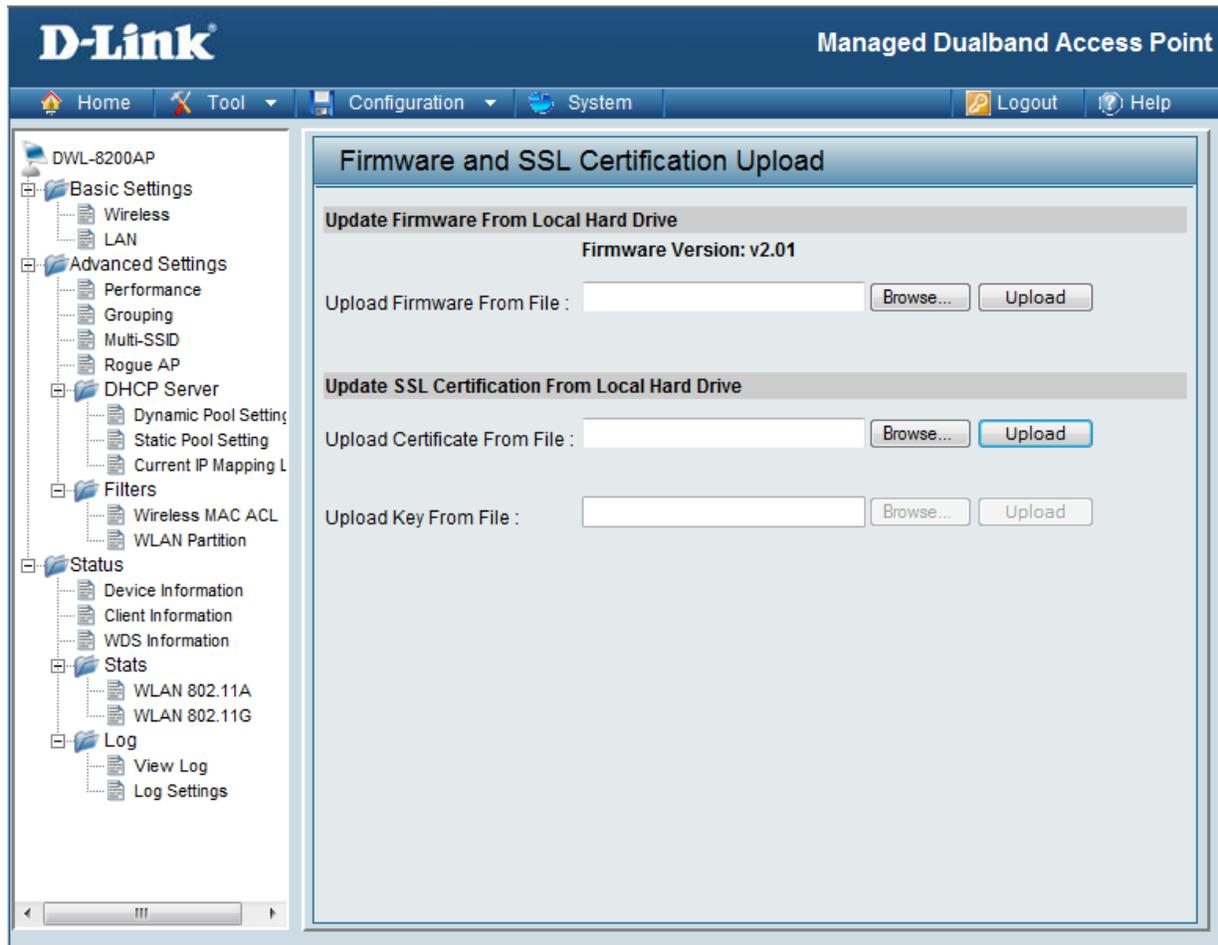
**Upload Firmware** After downloading the most recent version of firmware for the DWL-8200AP from <http://support.dlink.com> to your local computer, use the **Browse** button to locate the firmware file on your computer. Click **Upload** to update the firmware version.
