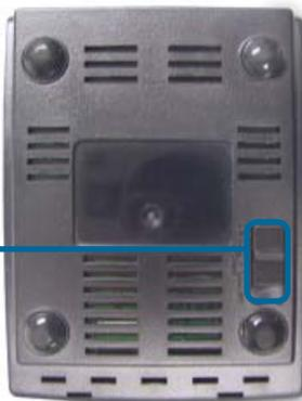
**Mode Selection Switch:** Used to select AP, client, or router mode.
