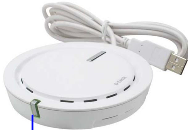
**Power LED:** A steady green light indicates that the WiMAX Adapter is ready for use.
