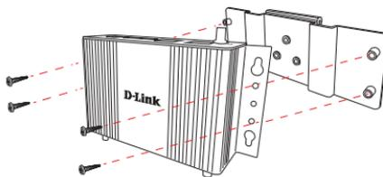
**Figure 7: Mounting the DIN Plate**
