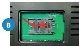
C. Slide the SIM card into the open tray with the gold contact points facing up.
