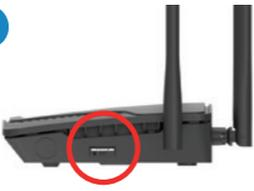
**B.** Slide the SIM card into the slot with the gold contact points facing upwards and the cut facing towards the router.
